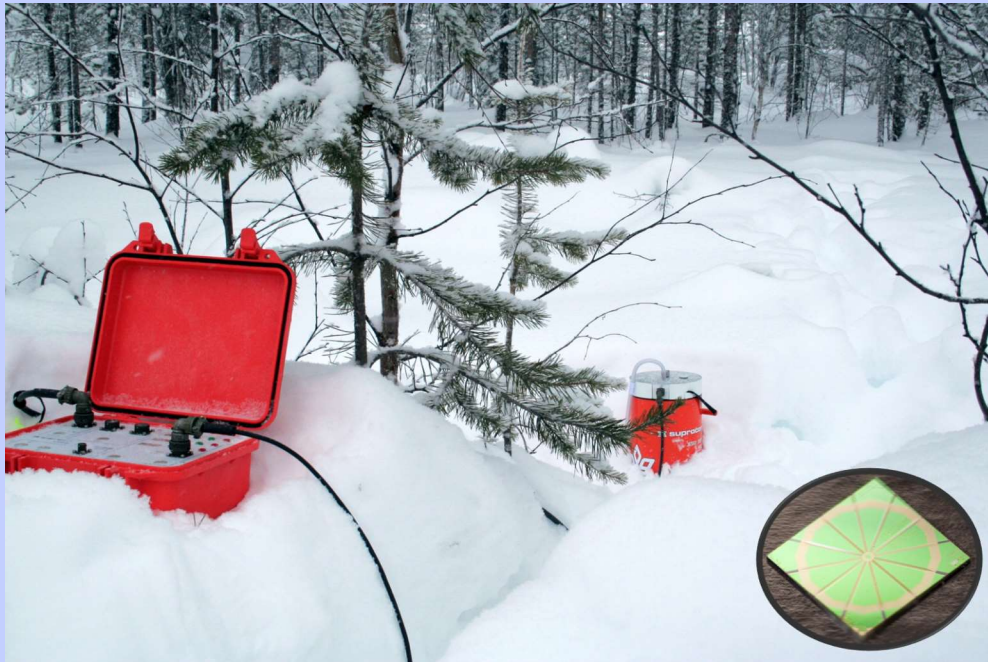
A SQUID magnetometer system in use on the field. The inset of the bottom right shows the superconducting SQUID chip where the loop that captures the magnetic flux is visible. Copyright: Leibniz IPHT and Supracon AG 2019.
